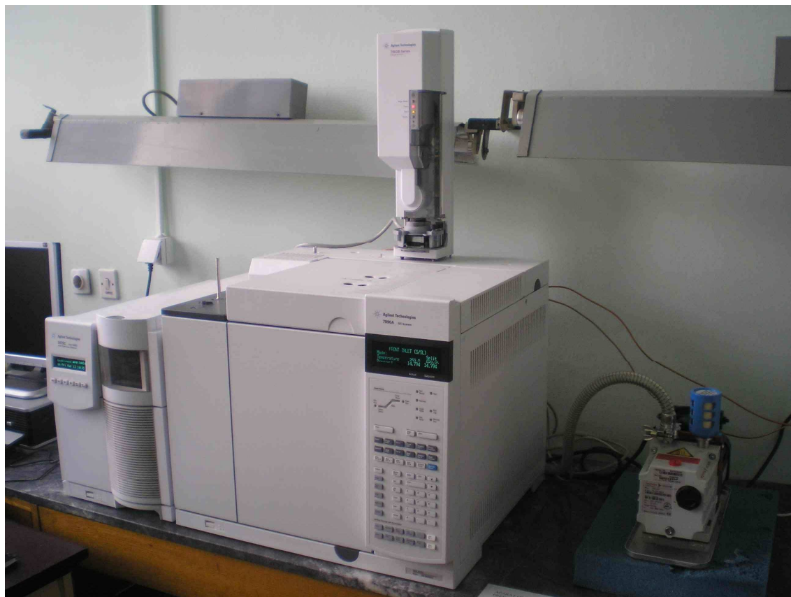
Figure 24. Gas chromatograph Agilent 7890N and a Hewlett-Packard 5972 MSD.
