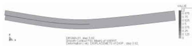
Fig. 20. Damage in matrix material when the maximum deflection has been reached
