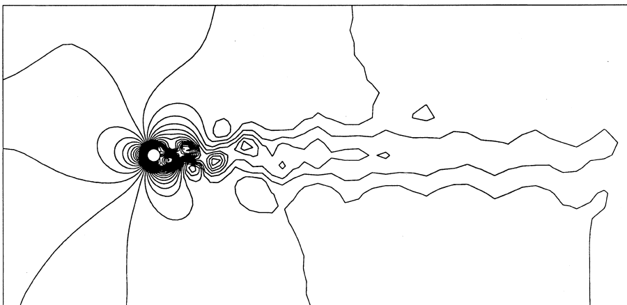
Fig. 17. Flow past a cylinder: pressure contours.
