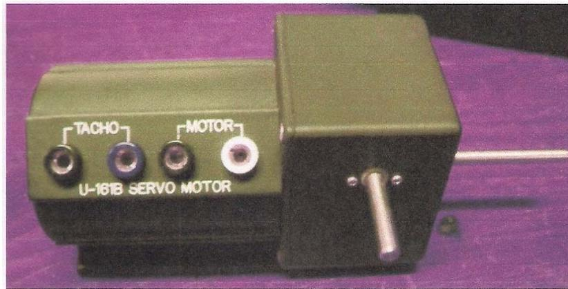
Gambar 3. Servo Motor
