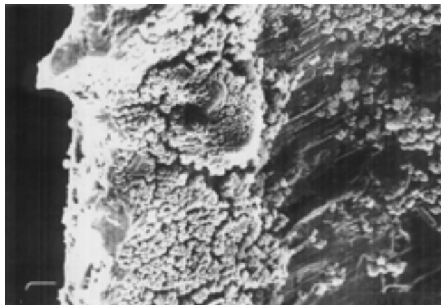
Figure 4. SEM microphotograph showing oral microorganisms colonies formed on a stainless steel band after 7 days of immersion. The border of the sample is clean showing that detachment of cells occurred during SEM pretreatments. Bar = 10 \mu\text{m} .
