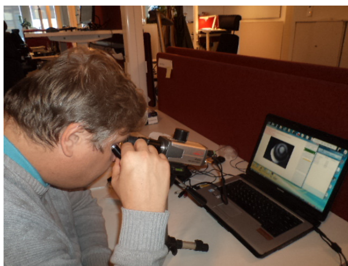
Fig. 3. The experimental model of the system for visualization of optical disk for practical illustration of structure of retina on the base of fundus system for eye observation FS 11
