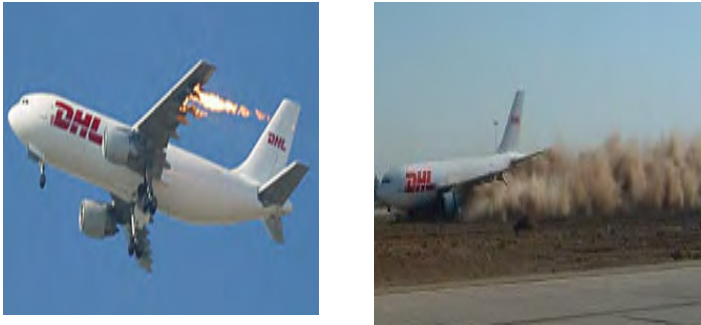
Fig. 1. Emergency landing sequence using engines only and left wing structural damage due to surface-to-air missile impact, DHL A300B4-203F, Baghdad, 2003
