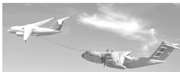
Fig. 1. The method of “inverse” air-to-air refueling
