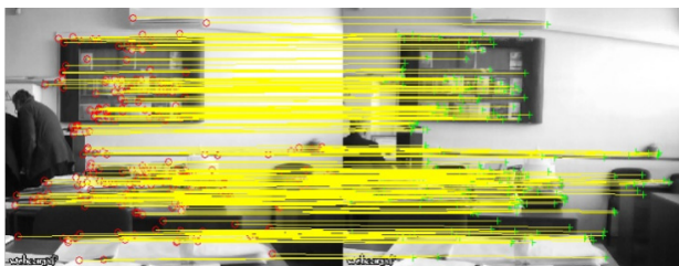
Fig. 2. Referenced image (left) and the same scene with camera rotation angle in 2^\circ . Matched points are shown by line connections. KLT tracker.
