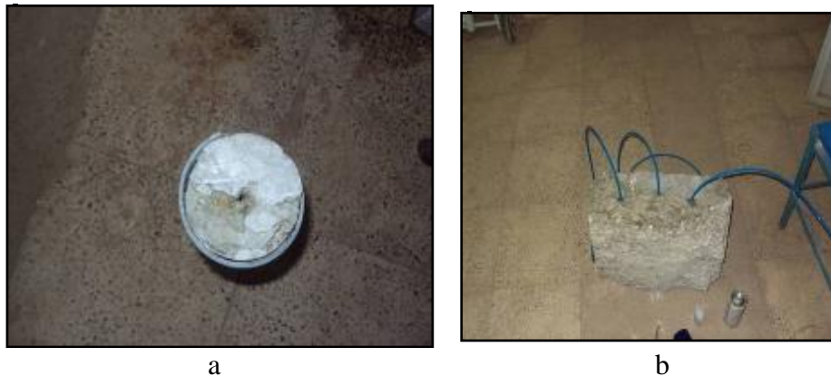
Figure 5: Piercing and preparation of gypsum specimens: a) cylindrical specimen, b) cubic specimens having 3 holes.
