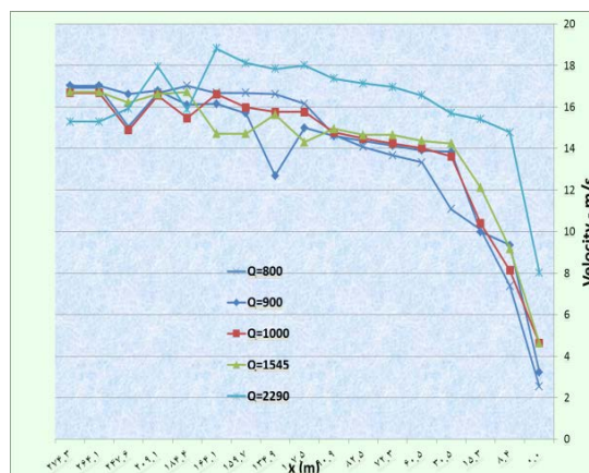
Comparing flow rate in different discharges with 90 cm height of steps
