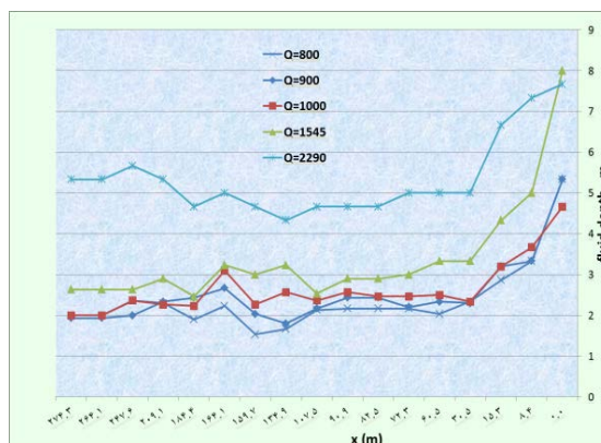
Comparing flowing depth in different discharges, with 90 cm height of the step
