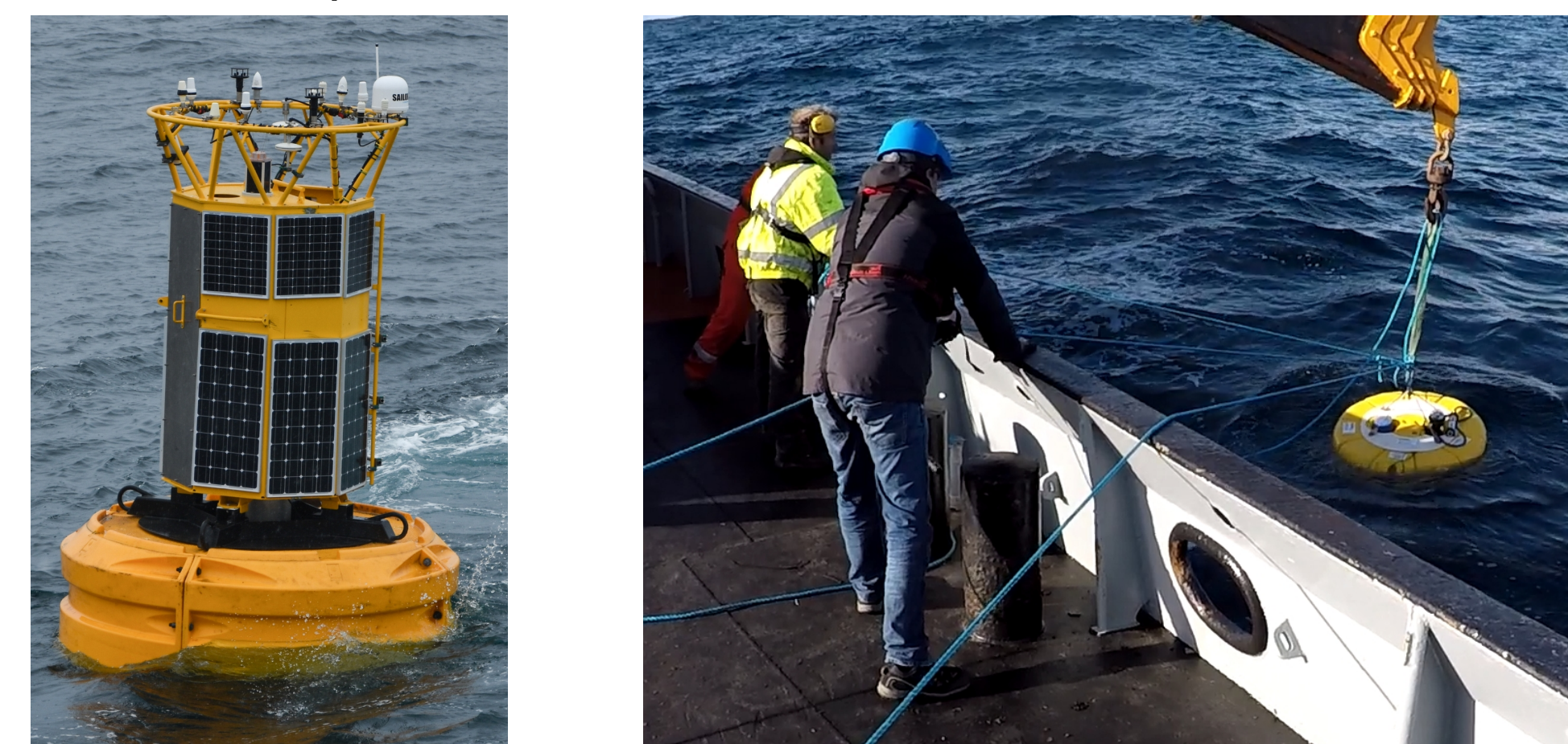
Left: The new M6 buoy which was deployed in June 2019 with the acoustic and satellite communication equipment for the OBS installed. Right: Guralp Aquarius+ been deployed in October 2019
