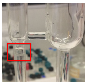
Figure 5. Close-up view of the extraction solvent recovery in a special homemade laboratory glassware.
