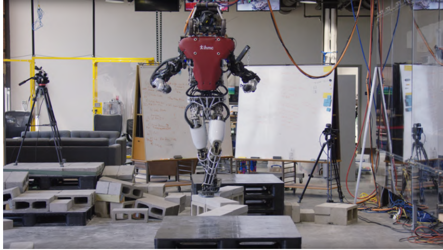
Fig. 1.7 The IHMC Atlas humanoid robot performing a complex walking task on top of a narrow cinder block pile.
