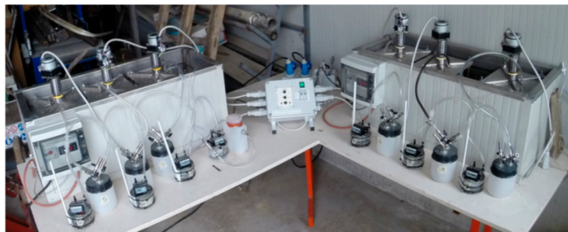
Figure 2. Detail of the experimental anaerobic digestion system.
