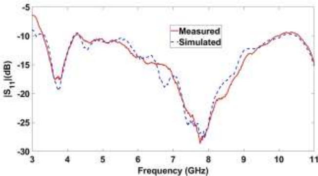
Fig. 3:  $S_{11}$  frequency response of the proposed PCMA.
