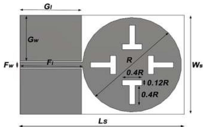
Fig. 1: Layout of the proposed PCMA.
