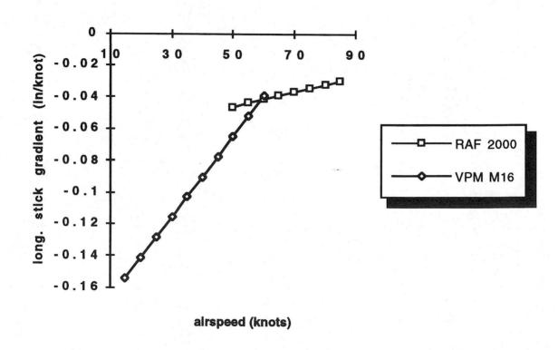
Figure 4 -- Comparison of stick position gradient with speed, RAF 2000 and VPM M16
