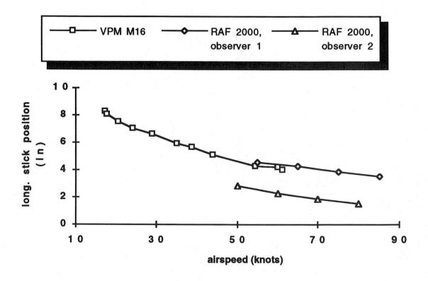
Figure 3 -- Comparison of stick position with speed, RAF 2000 and VPM M16
