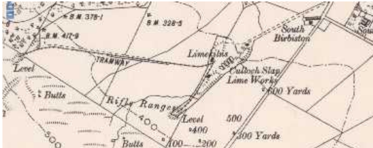
Figure 11. OS 2nd edition 6" mapping of Culloch Slap lime works showing rebuilt lines and new tramway (Stirlingshire Sheet 27. Surveyed 1896, published 1899). The elevated ridge that carried this second tramway is still clear in the field. (Reproduced by permission of the National Library of Scotland)
