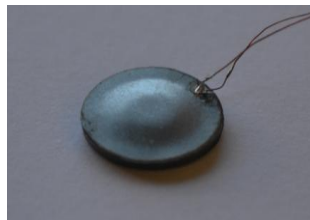
Fig. 1. A fully-assembled Nitinol cymbal transducer.
