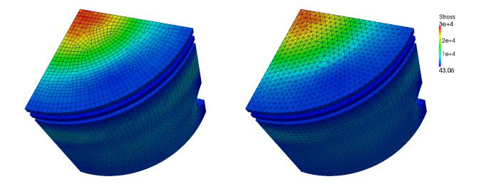
Figure 13: Mapping of stresses (using the element shape function). The source mesh (left) has 9,387 hexahedron elements, while the target mesh (right) has 28,635 tetrahedron elements.
