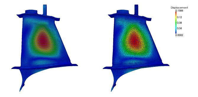
Figure 12: Mapping of displacements (using the element shape function). The source mesh (left) has 83,316 tetrahedron elements, while the target mesh (right) has 154,407 tetrahedron elements.
