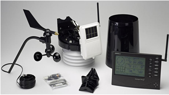
Figure 6: Davis Vantage Pro 2 weather station with anemometer, solar panel and wireless transmitter, radiation shield with air temperature sensor, rain collector, and indoor console davisnet: 2013
