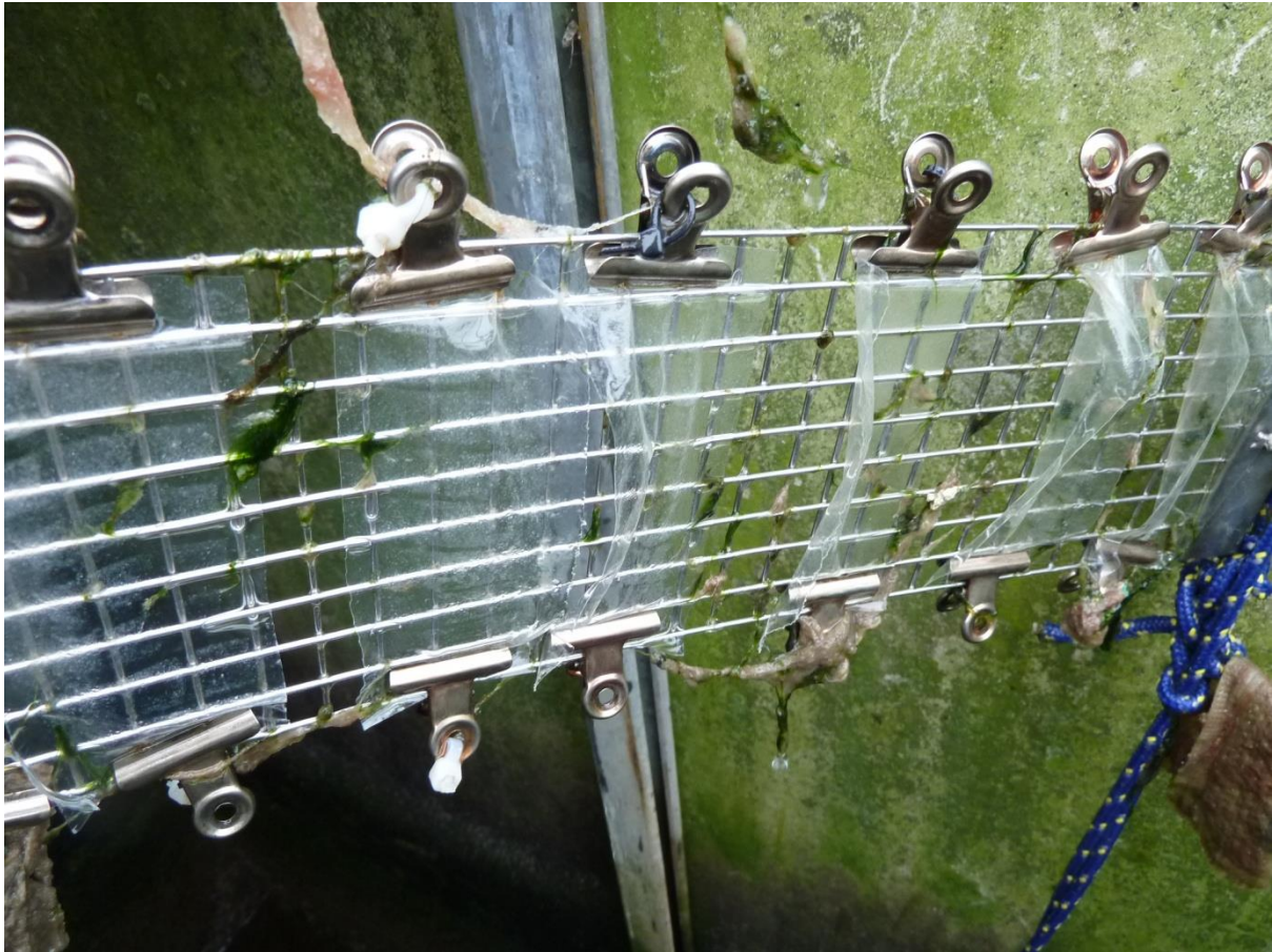
Fig. S5. Set of LDPE membranes at the end of the field trial. Due to the highly turbulent conditions in the waste water effluent channel even after deployment for one week there was minimal biofouling of the surface the membranes.
