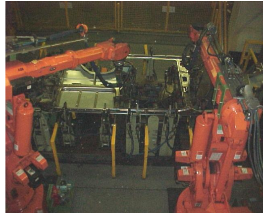
Fig. 2. Spot-welding process being performed by industrial robots.
