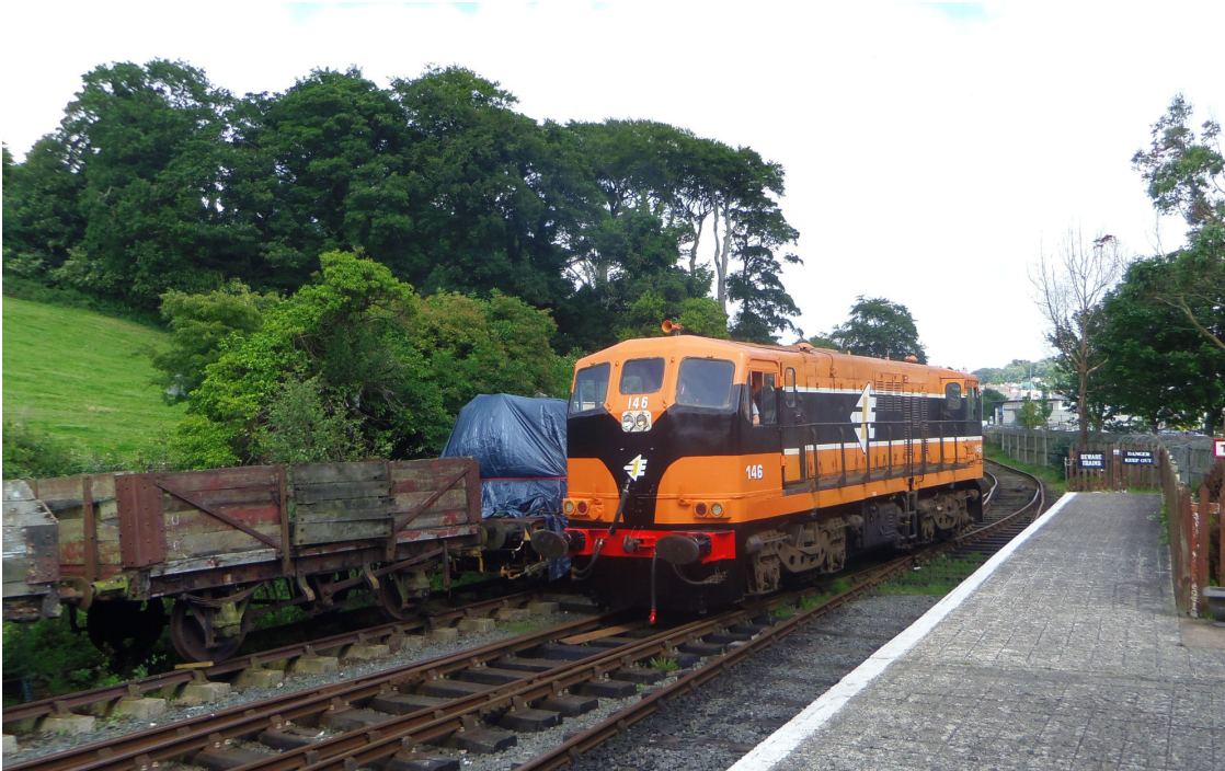
Running round, ex CIE 141 (B) Class Bo-Bo Locomotive 146, 1962 General Motors 0-4-4-0 locomotive at Downpatrick, 4 August 2012.
