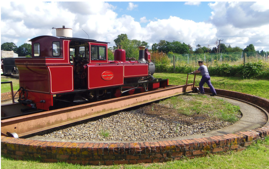
Bure Valley Railway, the engine driver rotates the turntable at Wroxham, 8 August 2012. The engine is the 15 inch gauge locomotive No. 9 'Mark Timothy' 2-6-4 Tank ZB Class. This was originally built by Winson Engineering as an oil fired loco, rebuilt by Alan Keef Limited as coal fired. It entered full service in July 2004.
