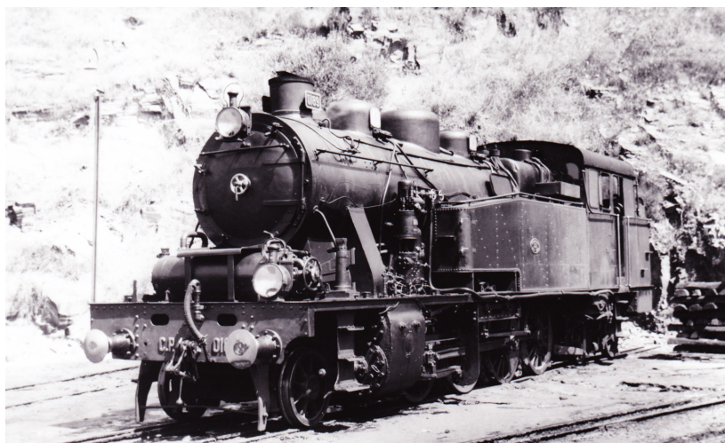
0189 2-8-4T Henschel 1925 Mallet locomotive at Regua.
