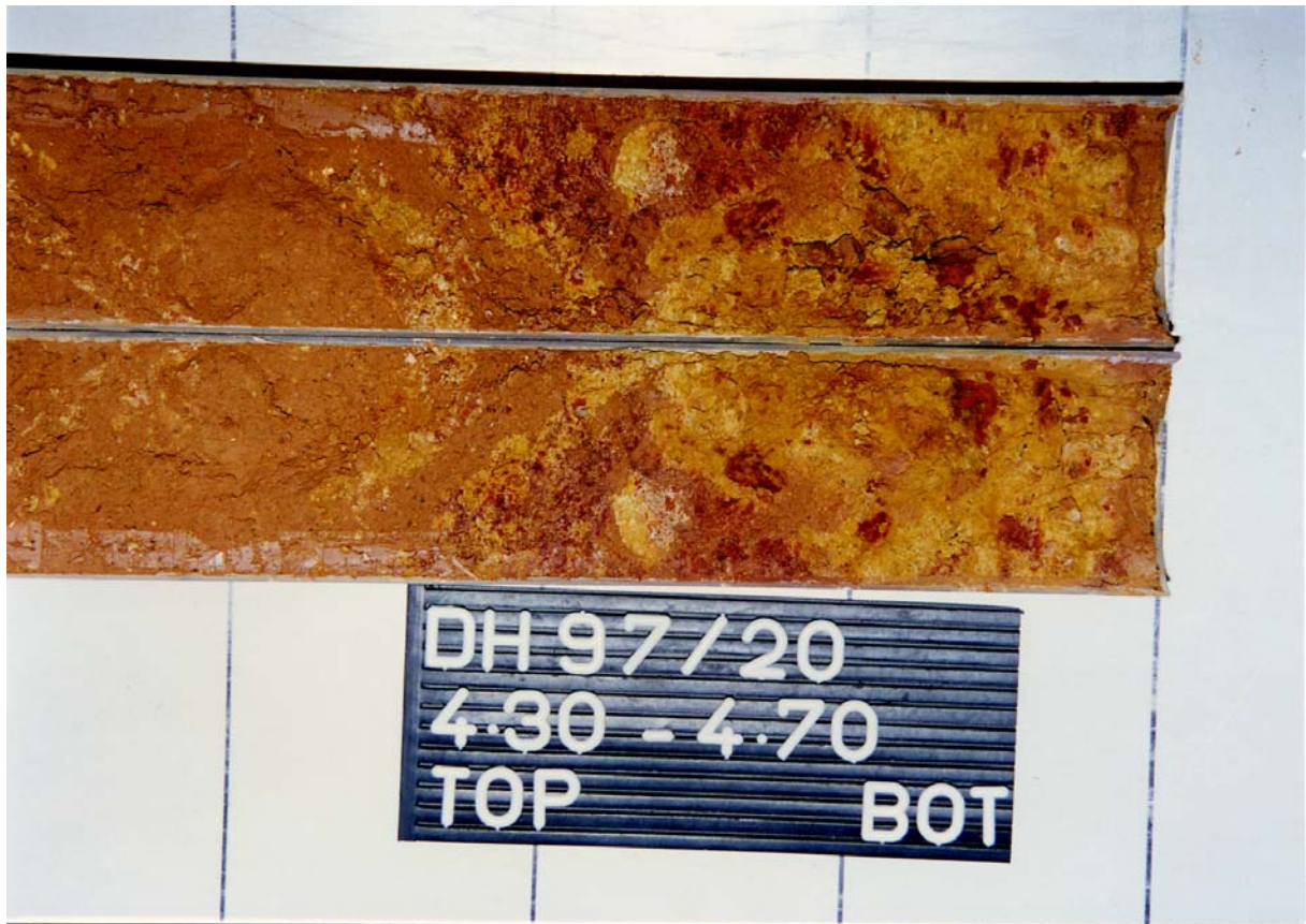
Plate B1 - Drillhole 97/20 - Split Maizier 4.30 m to 4.70 m Transition Zone from Residual Soil into Saprolite.
