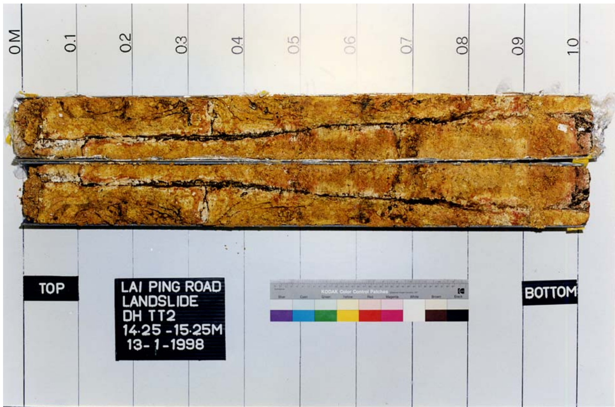
Plate B3 - Drillhole TT2 - Split 4CMLC Core 14.25 m to 15.25 m. Typical Sub-vertical Joint in Completely Decomposed Tuff.
