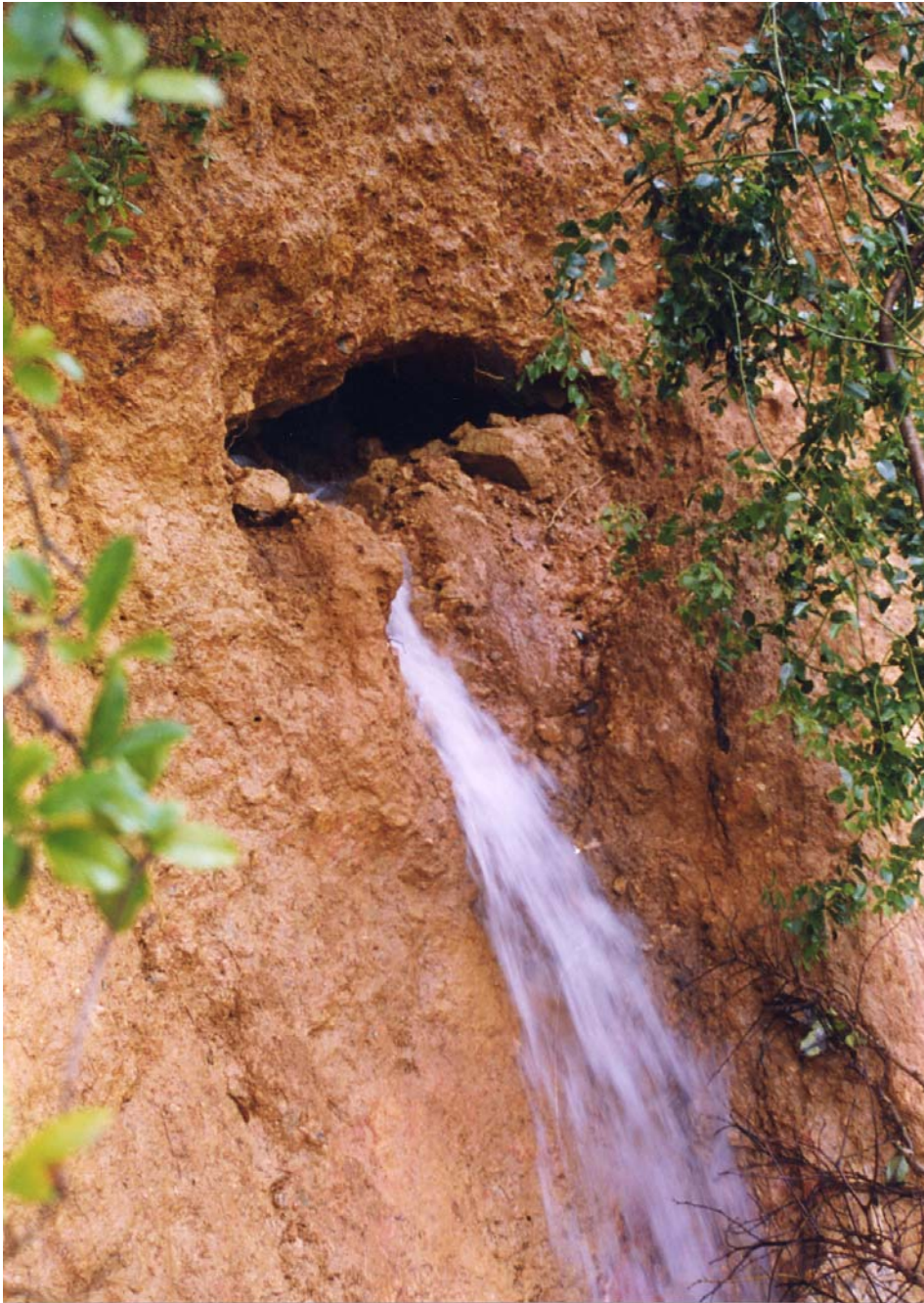
Plate 28(c) - Soil Pipe with Heavy Flow (Plate Location Shown on Drawing EG503) (Taken on 9/9/97)
