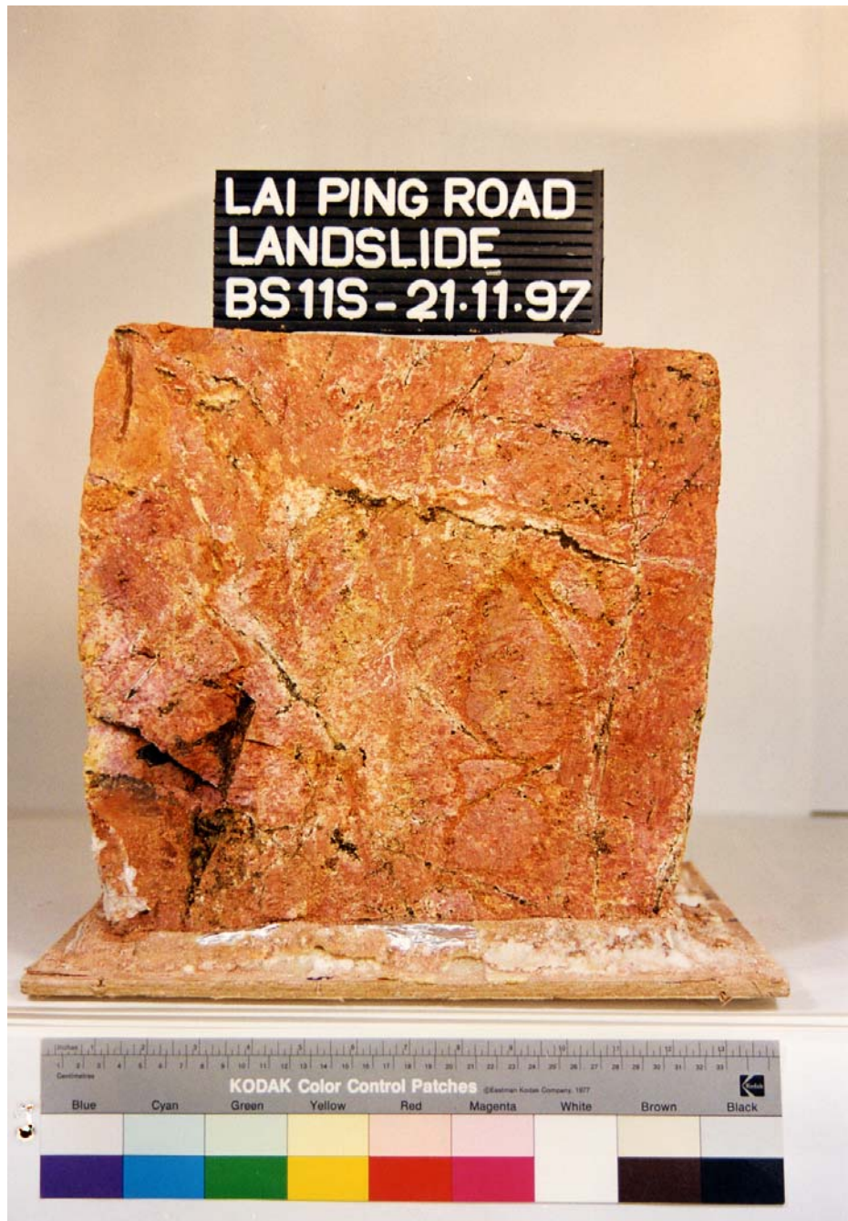
Plate 7(b) - Southern Face of Block Sample 11 - Intensely Altered Tuff - Note Contorted Relict Joints Infilled with White Kaolin and Manganiferous Deposits (Plate Location Shown on Drawing EG503) (Taken on 21/11/97)
