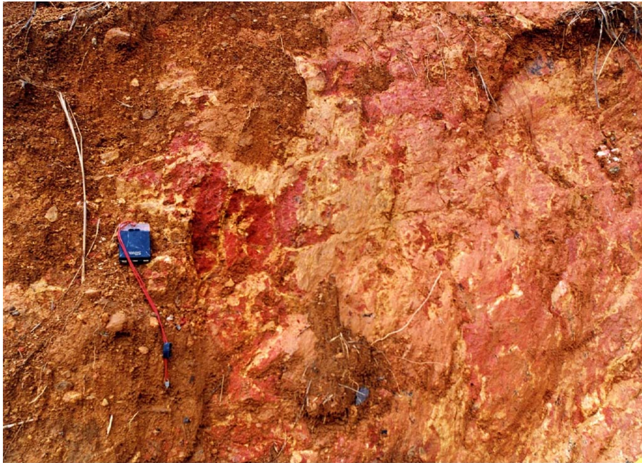
Plate 7(a) - Intensely Altered Coarse Ash Crystal Tuff Exposed in Landslide Scar 4A (Plate Location Shown on Drawing EG503) (Taken on 6/8/97)
