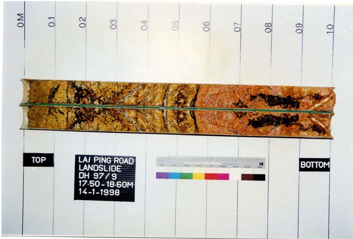
Plate B4 - Drillhole DH 97/9 - Split Maizier 17.50 m to 18.60 m. Sharp Junction between Completely Decomposed Tuff and Highly Altered Completely Decomposed Tuff.
