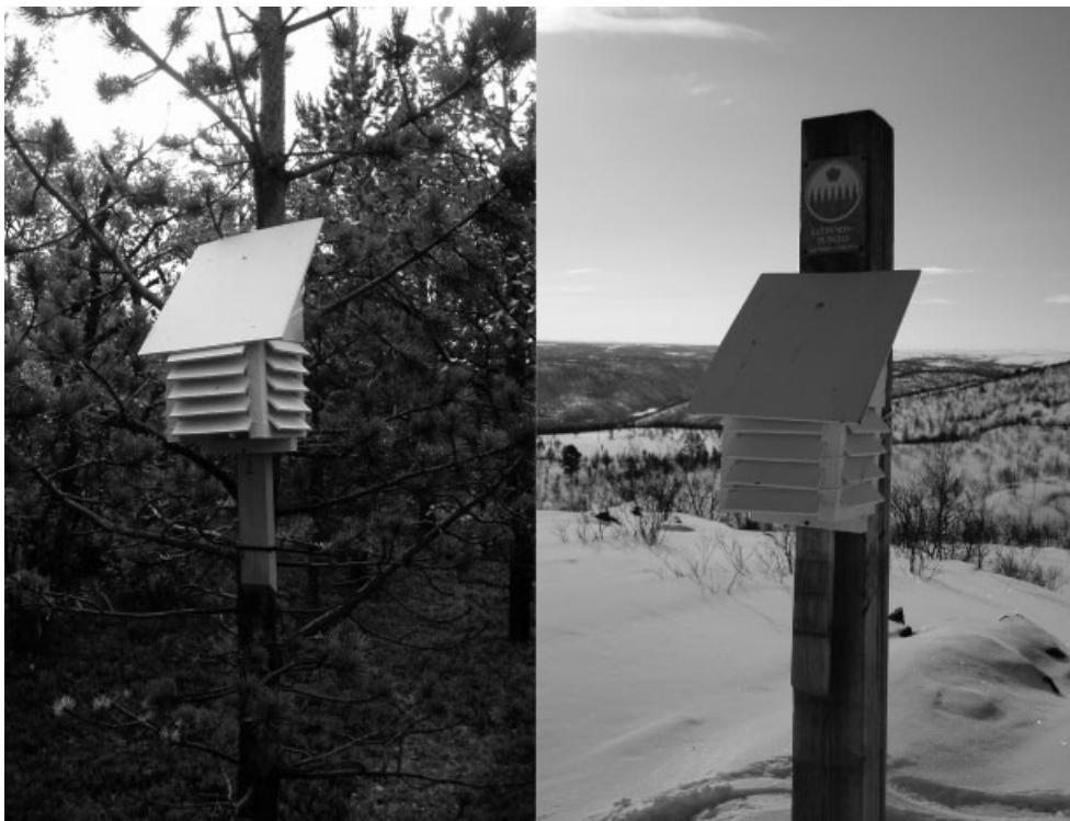
Figure 2. Temperature dataloggers housed in Stevenson screens and installed at 1.5 m above ground level below the treeline (left) and above the treeline (right).
