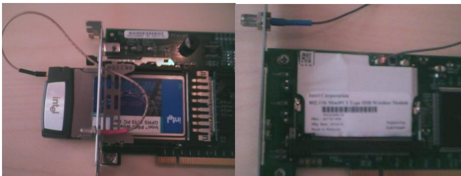
Figure 3 - Intel PRO/Wireless GPRS 3110 PC Card with Orange SIM card and Intel PRO/Wireless LAN 2100 3B MiniPCI Adapter.
