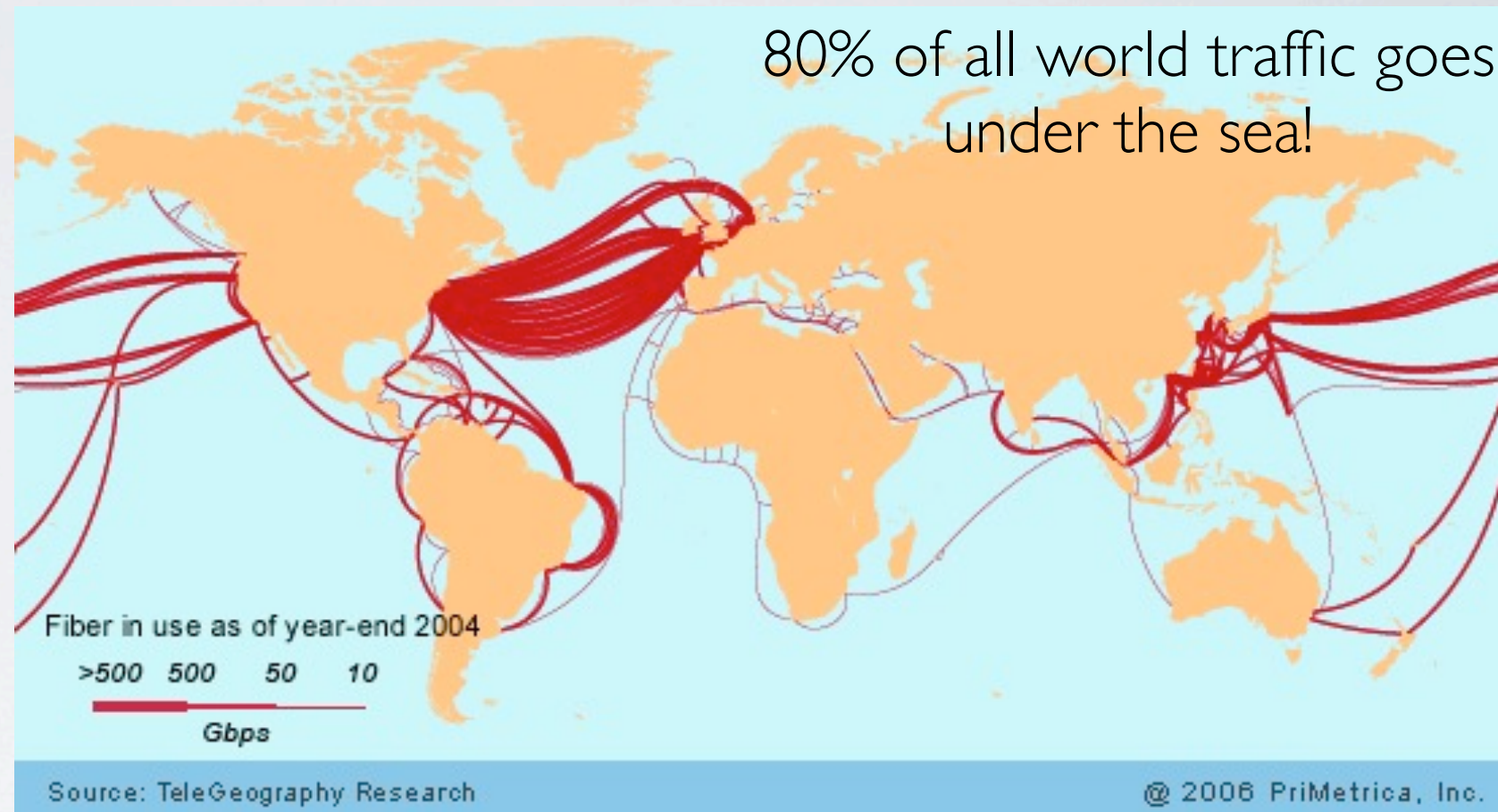
fiber optics under sea cables (internet backbone)
