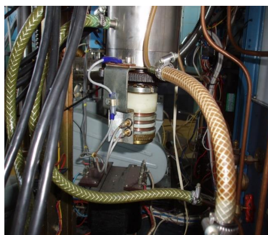
Fig. 1 Parts of the HF CVD system below the vacuum jar. One can see the rotary mechanism, sliding annular contacts, outputs of the thermocouples (grey cables) and temperature compensation (blue connection).
