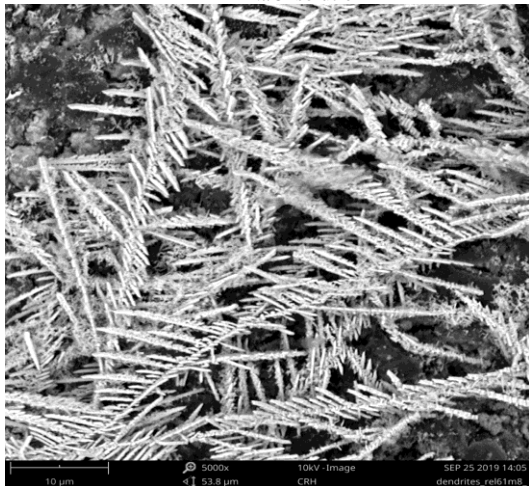
Fig. 13. SEM micrography of the dendrite of solder paste REL61 in 2mM NaCl solution
