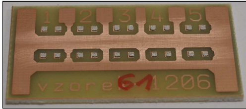
Figure 2. PCB with applied electrically conductive adhesive.
