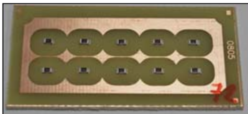
Figure 3. PCB with placed 0805 chip components.
