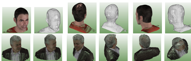
Figure 7: Results of the entire pipeline. First row: several views of the point cloud and carved volume obtained from VH and four multiscopic units for virtual actor "Simon". Second row: several views of the global point cloud obtained for real actor "Jacques" from final volume resulting from VH and three multiscopic units. It corresponds to the union of the projection, per multiscopic unit, of the initial point cloud on the final volume.
