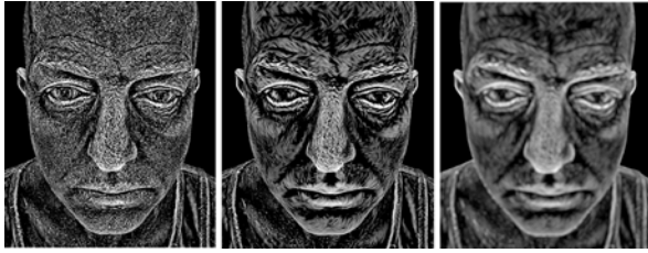
Figure 7: Using the normal map to compute the screen space curvature results in a noisier curvature (left). Geometry normals reduce the noise (center). We smooth this map to feed the algorithm with a smoother curvature map (right) free of high frequency discontinuities.
