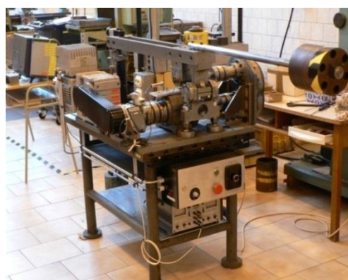
Figure 1 – Measurement of contact path width (left) and TUORS II twin-disc experimental rig (right)
