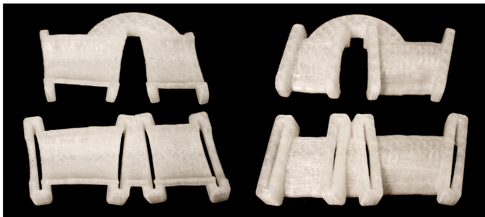
Figure 8: Fibula cutting guide models 3D printed in polyactide (PLA) plastic.
