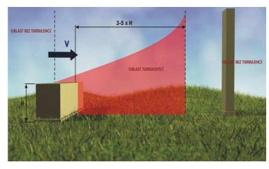
height, so rotor near the barrier must be placed higher in order not to be subjected to beats and vibration whereby financial demands of construction of the power plant body tube grow up. The influence of turbulence becomes weak with the growing distance from the barrier.
