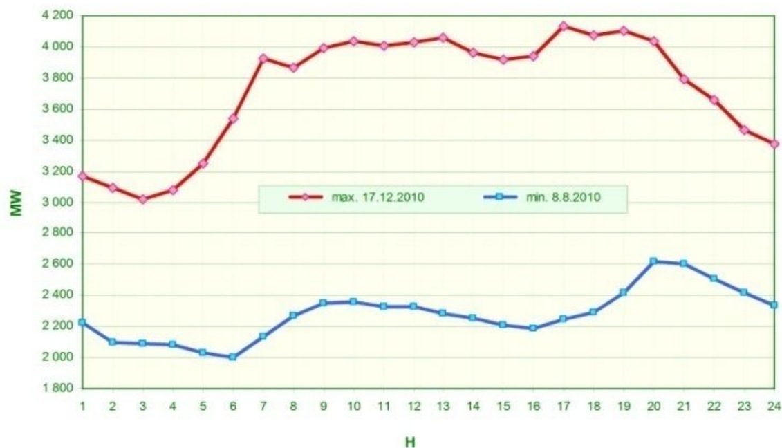
Figure 2 - Daily load diagram for minimum and maximum year's load
