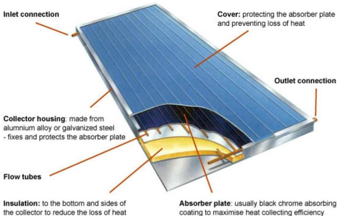
Figure 2 – Flat plate collector [3]
