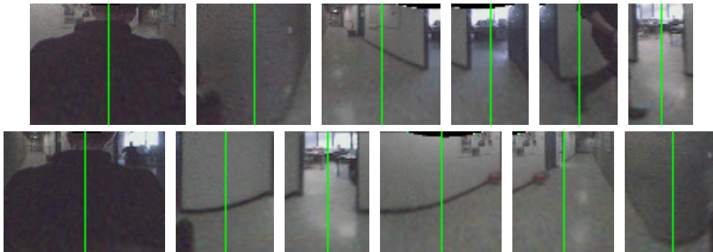
Figure 10: First level symmetry hierarchy of the panoramic images presented above. Top: sectors A_1 - A_6 . Bottom: sectors B_1 - B_6 . The proposed algorithm divides the images into highly symmetric segments.
