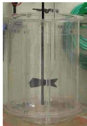
Figure 1: Stir Tank (Courtesy Dow Chemicals)
