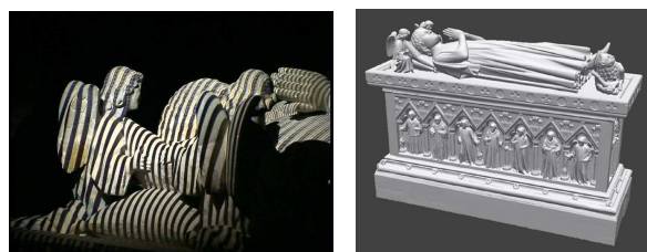
Figure 3: (left) 3D digitization using structured natural white light. (right) 3D colorless model displayed with Catia software (Dassault System).
