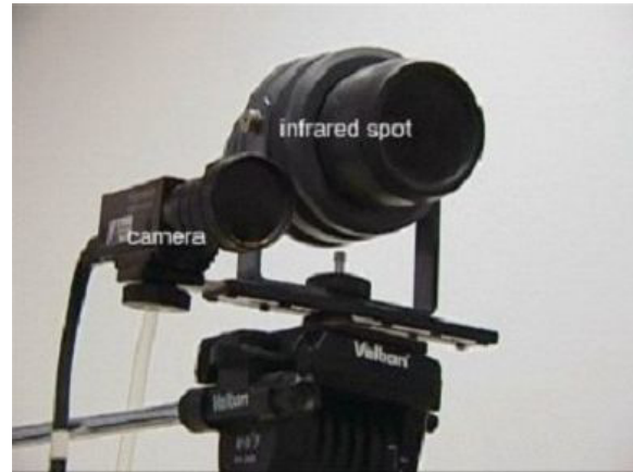
Figure 1: Camera and (optional) infrared light beamer
