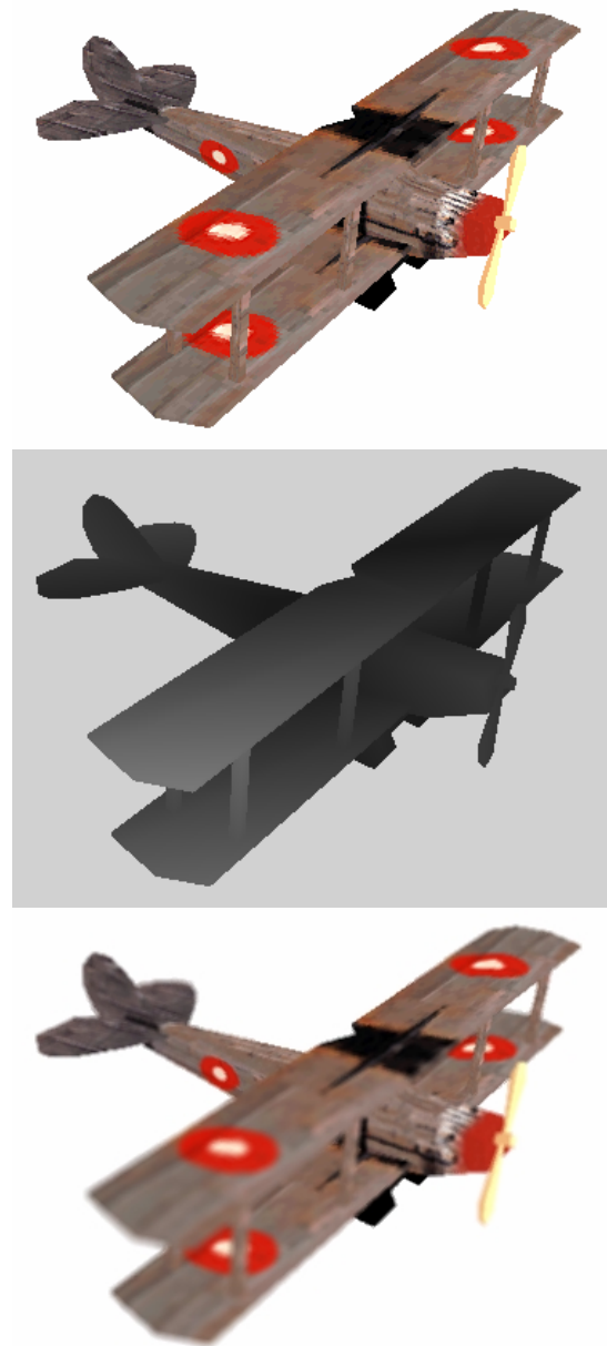
Figure 14. Examples of Depth of Field algorithm. Original, CoCs size and final images.
