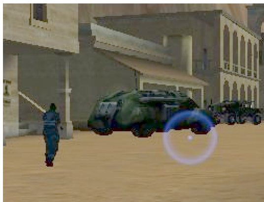
Figure 1. Example of blur chaos (screenshot from an FPS game). Soldier and tank looks like in the air due to poor texture anisotropic filter and sharp triangle edges.
