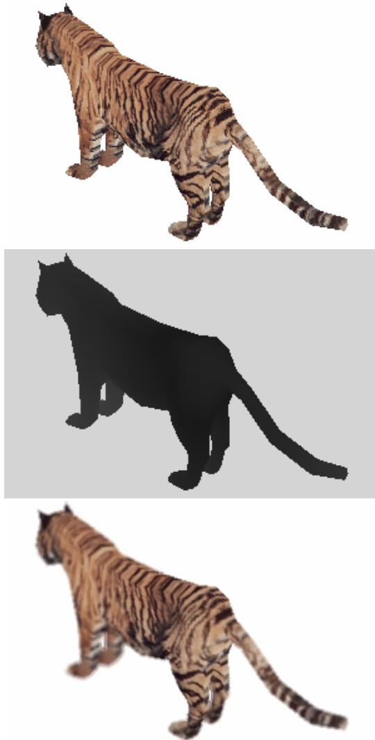
Figure 13. Examples of Depth of Field algorithm. Original, CoCs size and final images.
