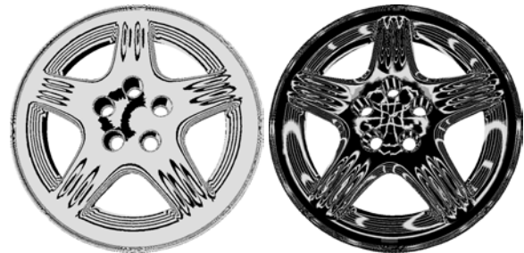
Figure 7. Wheel rim rendered with isophotes and reflection lines
