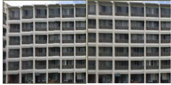
Figure 7 – Refining texture alignment. Left: texture painting using only 3D model based warping, which results in significant misalignment due to inaccurate camera pose. Right: texture painting after refining the texture alignment.
