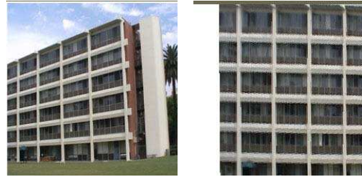
Figure 3 - Result of the model based image warping. Left: original image, right: image warped to base buffer.
