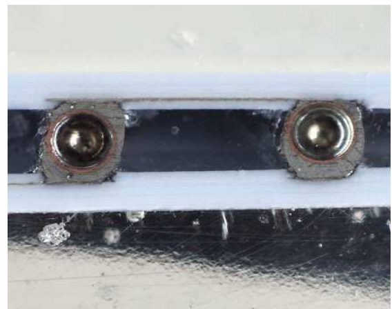
Fig. 5: Micro sections of solder joints with Sekisui SOL balls
