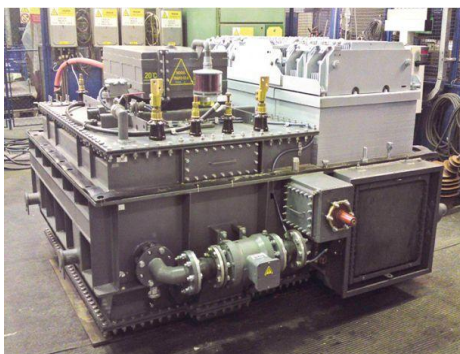
Fig. 2: Railway traction transformer prototype. Type T1T-4900-25/2x1700 [2]
