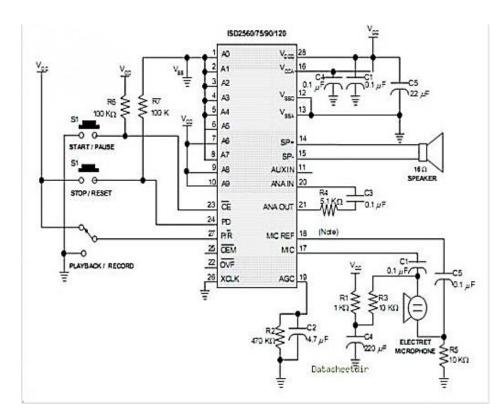
Figure 7. ISD25120 sound recorder IC
