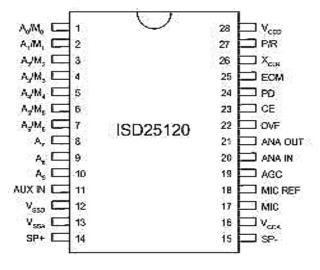
Figure 4. ISD25120 device pinouts
