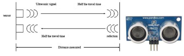
Figure 2. How ultrasonic sensors work [22-24]
