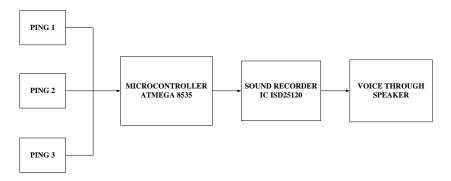
Figure 5. Block diagram of the system tool design
