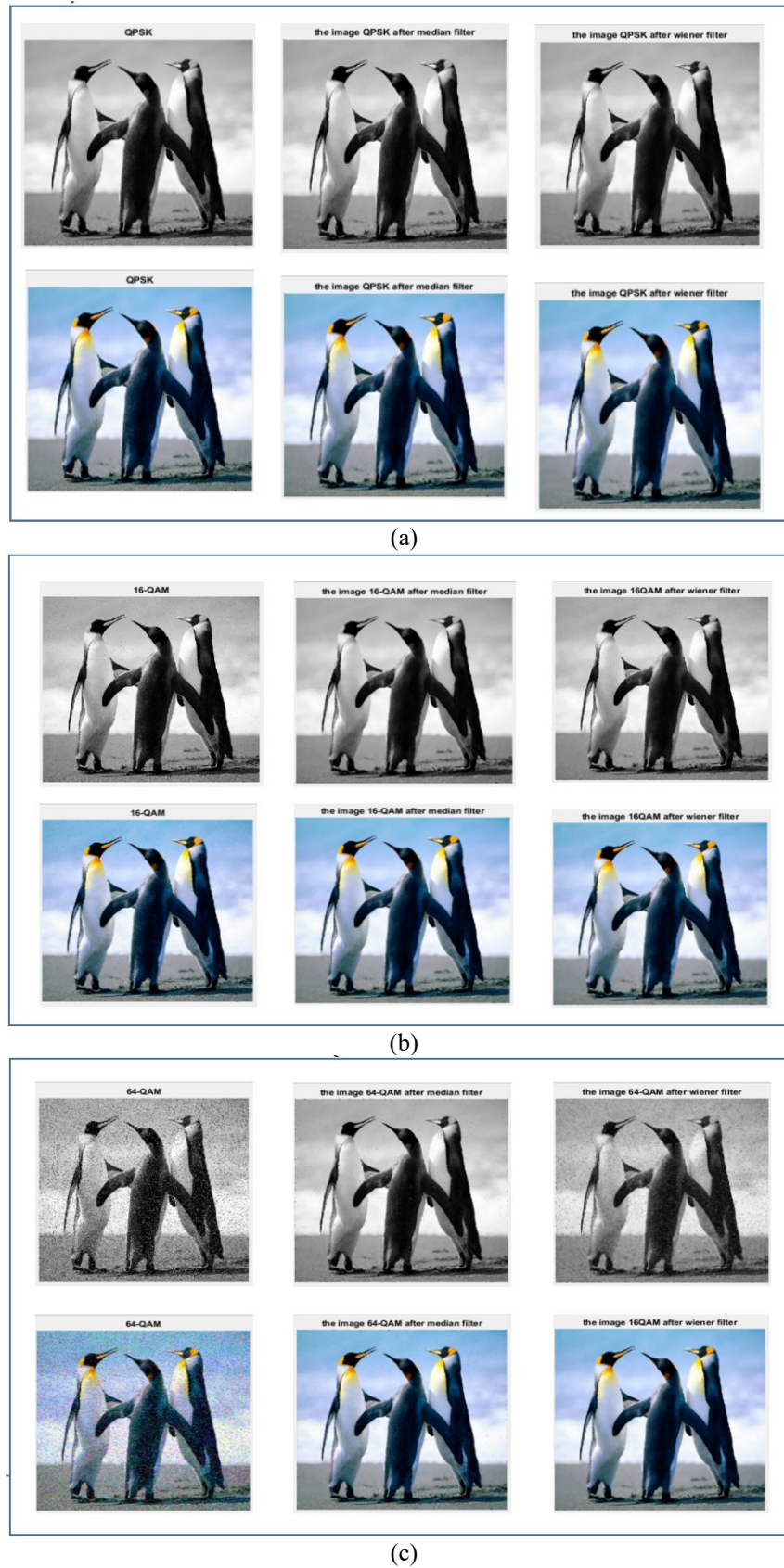
Figure 2. Comparison of recovered images at the system receiver without filter, with median filter and with wiener filter for different modulation schemes over AWGN channel; (a) QPSK modulation scheme, (b) 16-QAM modulation scheme, and (c) 64-QAM modulation scheme
