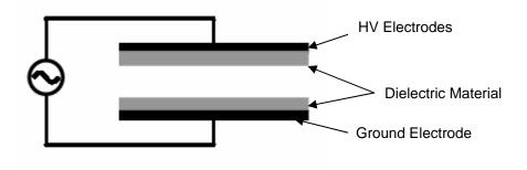
Figure.1 The basic configuration of ozone generation
